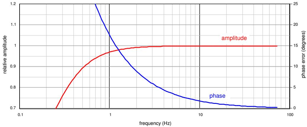
A good low-frequency response is useful when monitoring power-frequency transients where the wave-form can have a 'DC offset' which lasts for a few cycles.
