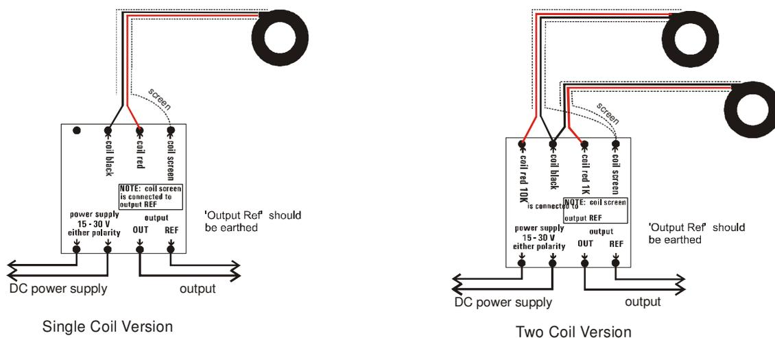
important. to ensure that the coils are connected in the correct phase relative to each other so that their contributions add rather than subtract (section 3.3). A dual-coil version can also be used with one coil only if needed. The other input should be left open-circuited.
