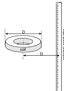
**INFLUENCE OF CONDUCTOR POSITION:** If the conductor is moved from the central position by a distance equal to 0.5 x the coil radius the output will change by less than 1%.
