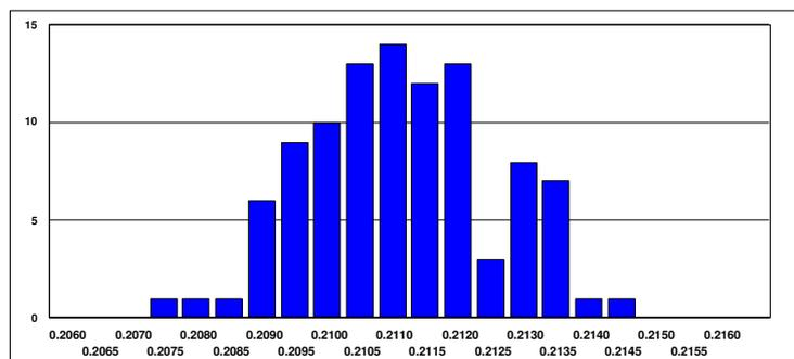
system) the integrator is adjusted to suit the coil. We also have an interchangeable coil system which can be used with appropriately-designed integrators. This allows coils to be replaced or interchanged between integrators without the need to re-calibrate the integrator. The figure shows the spread in mutual inductance values for a batch of 100 Type 1012 coils manufactured at the same time.
