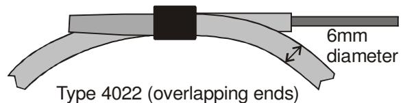
4022: Unscreened coil with a plastic clip to locate the ends as in the picture at the start of this memo. This coil is most suitable for situations where the coil is to be moved around to different locations.
