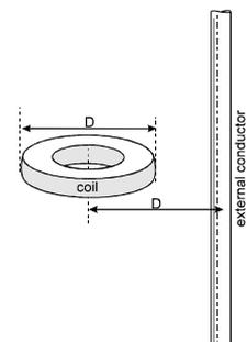
**INFLUENCE OF CONDUCTOR POSITION:** If the conductor is moved from the central position by a distance equal to 0.5 x the coil radius the output will change by less than 1%.
