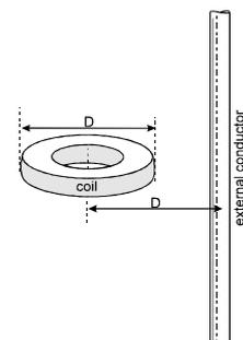
These tests are carried out on each coil at several stages during its construction. The information is used to make small adjustments to the winding to 'fine-tune' it for minimum pick-up. After the winding has been
