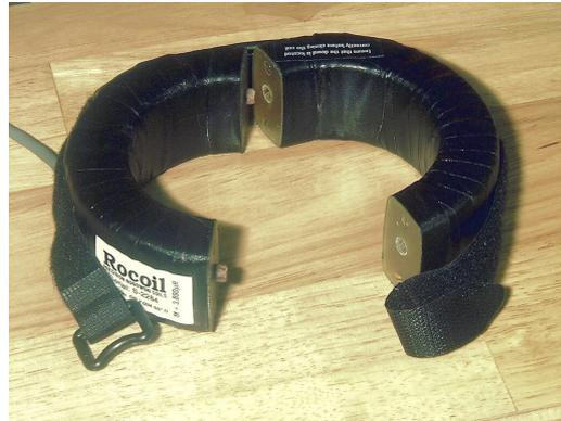
Rogowski Coils are much less sensitive to misalignment than conventional split current transformers. With an SX-76 coil, for example, a gap error of 0.3mm would introduce an output error of less than 0.1%. The phase is not affected even by a much larger gap.
